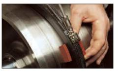
Stage 3: Clamp in position with steel band.
