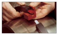
Stage 2: Align joint in moulded jig.
